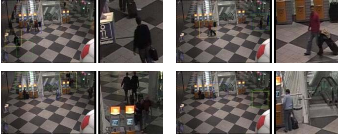
Figure 8: Four typical frames from an airport surveillance video, with three trajectories and fixed window size. In each frame, the original video frame, showing the locations of the cropping windows, is to the left and the cropped frame is to the right, resized to the original's height.
